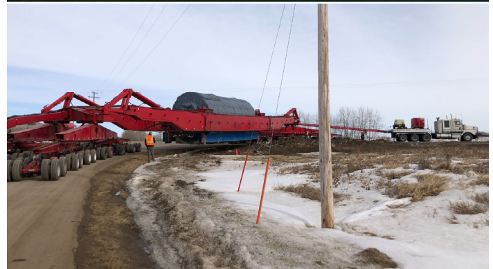
Top: Stormwater pond (foreground); erection of structural steel for generation building (background). Above: Delivery of Unit 20 generator to site
